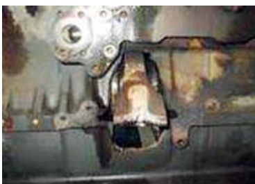
Big end bearing failure
