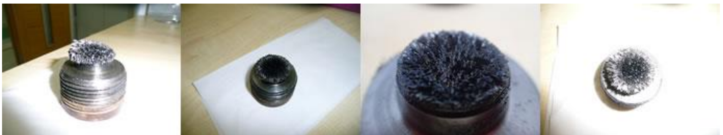
Damaged magnetic plugs showing excessive wear
